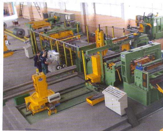
A good example: Slitting line for mild and carbon steel, installed in Ukraine
